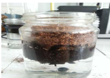
Fig. 9. The behavior of peat moss in water and REBCO.
