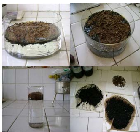
Fig. 5. Mixture of REBCO, water and peat moss.
