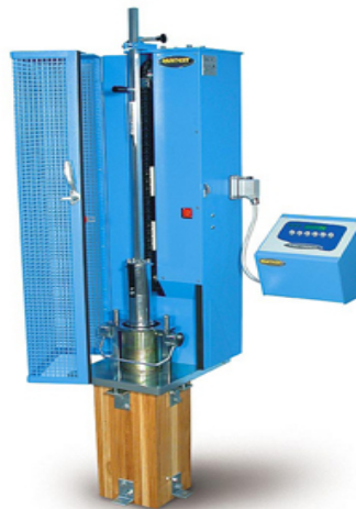
Fig.2. The pile driver Marshall for the manufacture of test specimens.
