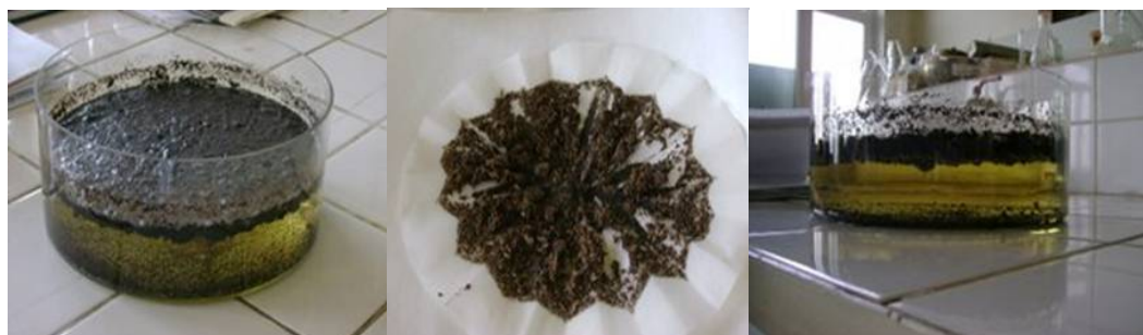
Fig. 7. Mixture of diesel, water and peat moss after 24 hours.
