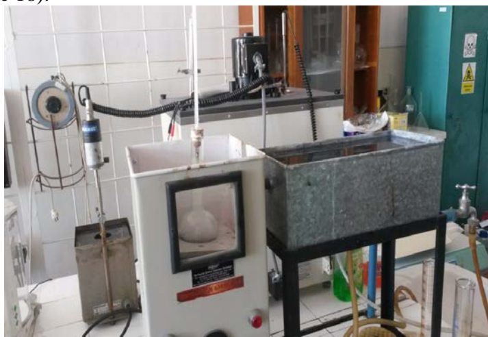
Fig. 18. The extraction of crude oil from sunflower seedcake soaked by Rebco crude oil
