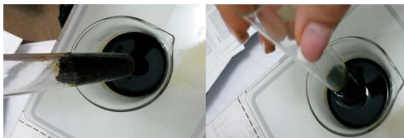
Fig. 14. The column used for tested the capillary ascension of sorbents
