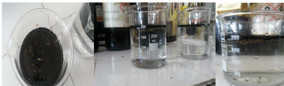
Fig. 21. The behaviour of sunflower seed cake in water and Rebco crude oil
