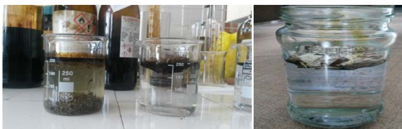
Fig. 22. Sunflower seed cake type 1 fails the test after 15 minutes
