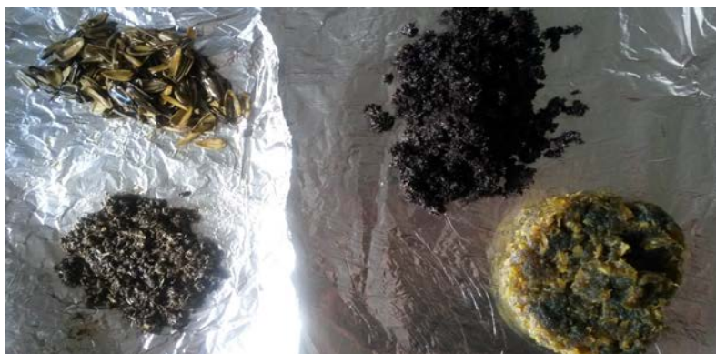
Fig. 12. The behaviour of the four sorbents analysed in contact with light vacuum oil
