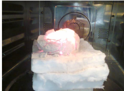
Fig. 3. The direct microwave heating test of the powder mixture based on waste glass
