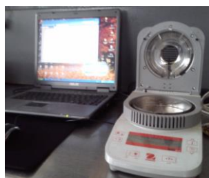
Fig. 2. Experimental setup for air drying of thin-layer vegetal material.
