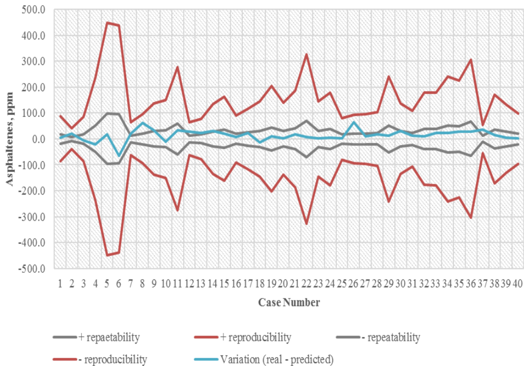
Fig. 5. State of repeatability, reproducibility and real predicted variation for cases from Fig. 3
