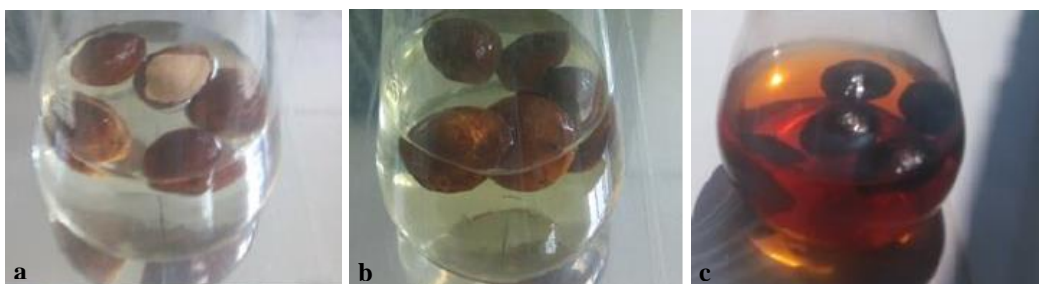
Fig. 3. System consisting of apricot stones and KOH solution after: (a) 1 min; (b) 10 min; (c) 2 h [16].
