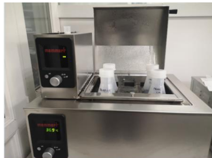
Fig. 4. The vessels with the studied samples, immersed in the solutions of artificial saliva with pH=2 and respectively pH=10
