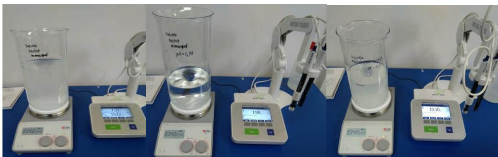
Fig. 2. Preparation of artificial saliva solution:left- with neutral pH; middle- with pH = 1.98; right- with pH = 10.
